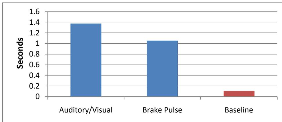
**Figure 15. Minimum time to collision for FCW systems**
