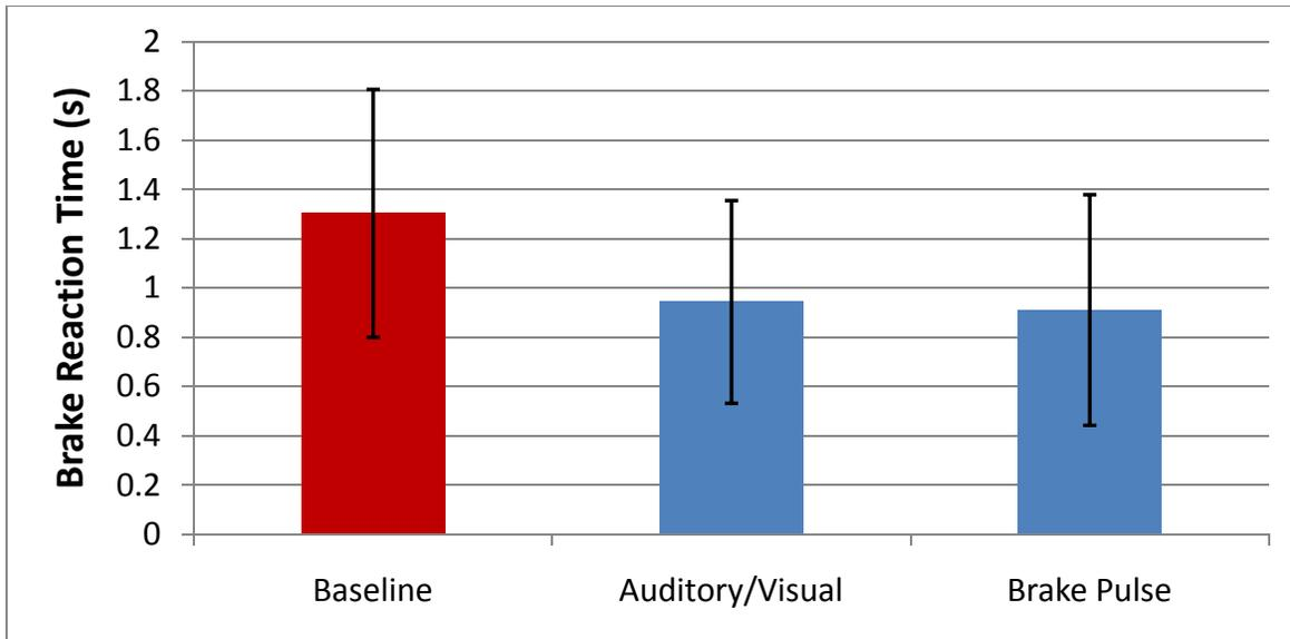
**Figure 4. Elapsed time between initiation of FCW alert and brake pedal pressed (with standard error bars)**
