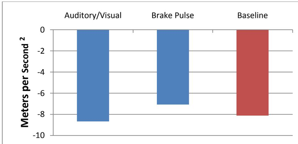
**Figure 14. Peak deceleration while braking for FCW systems**
