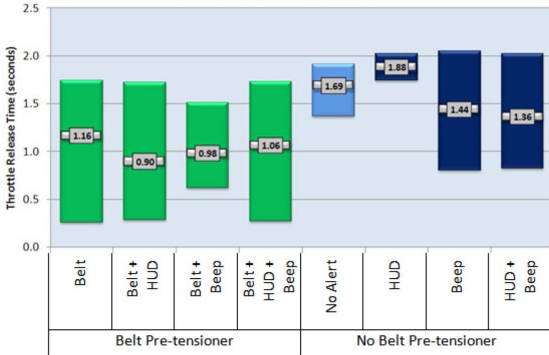
Figure 12. Throttle release times for FCW systems
